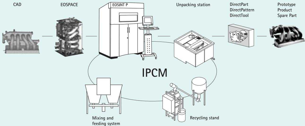
EOSINT P Process chain and IPCM. The ideal solution for the integration into an industrial environment.
